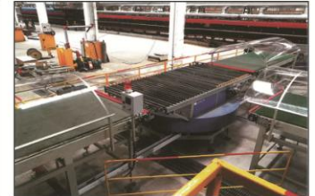
90° 托轮式转弯机 Wheel-Type 90° Curve Unit
